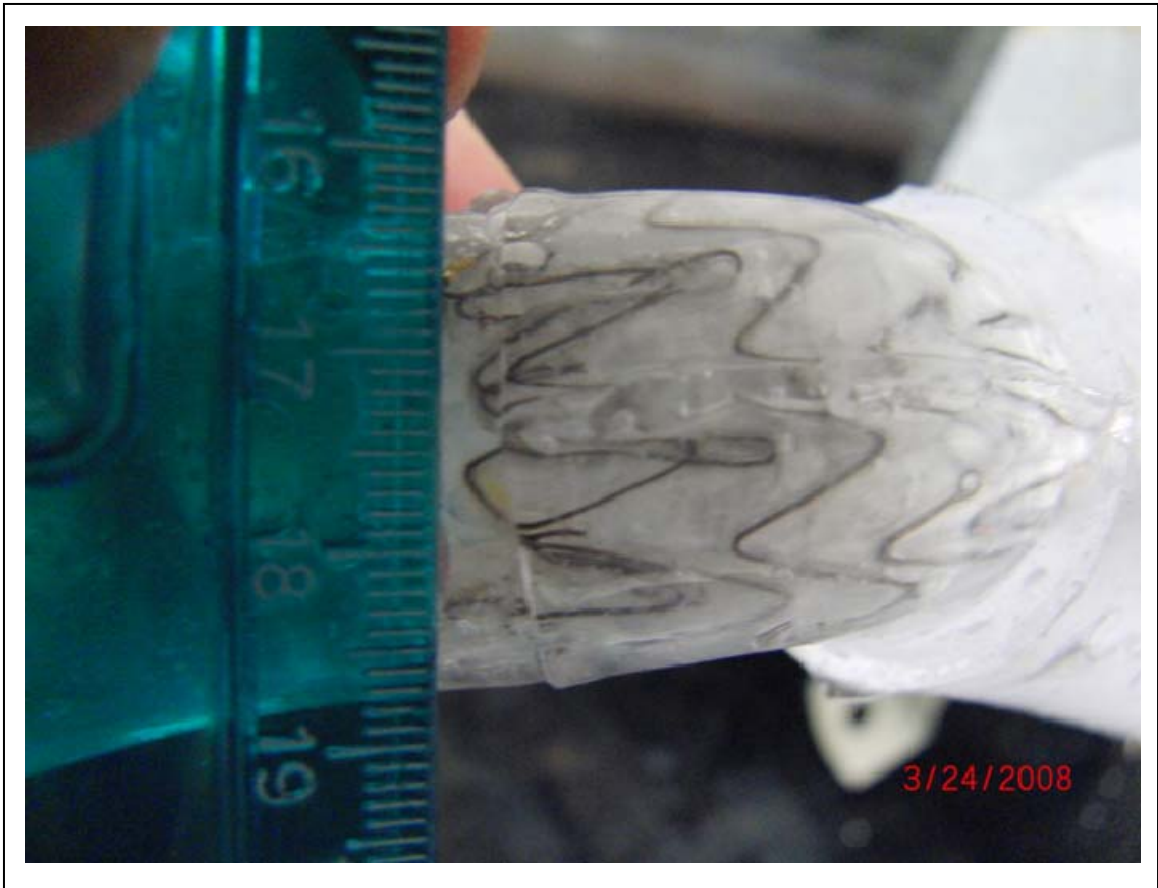
Figure 33: Folding and overlap of endograft stent struts at outer radius of the 60° neck angle bend.
