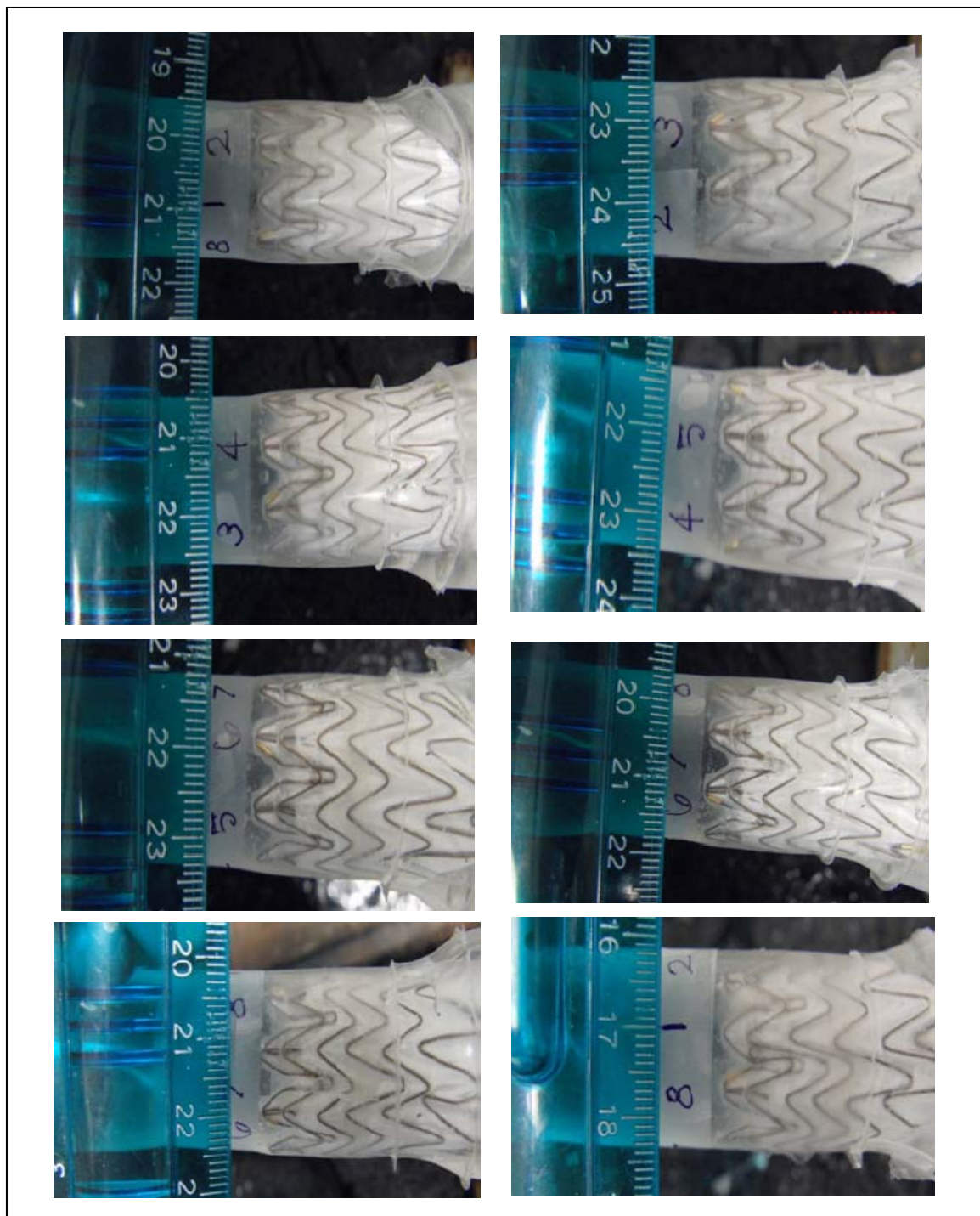
Figure 34: Representative images of apex to apex stent behavior throughout entire EVG perimeter for 0^\circ neck angle, 12% oversizing.
