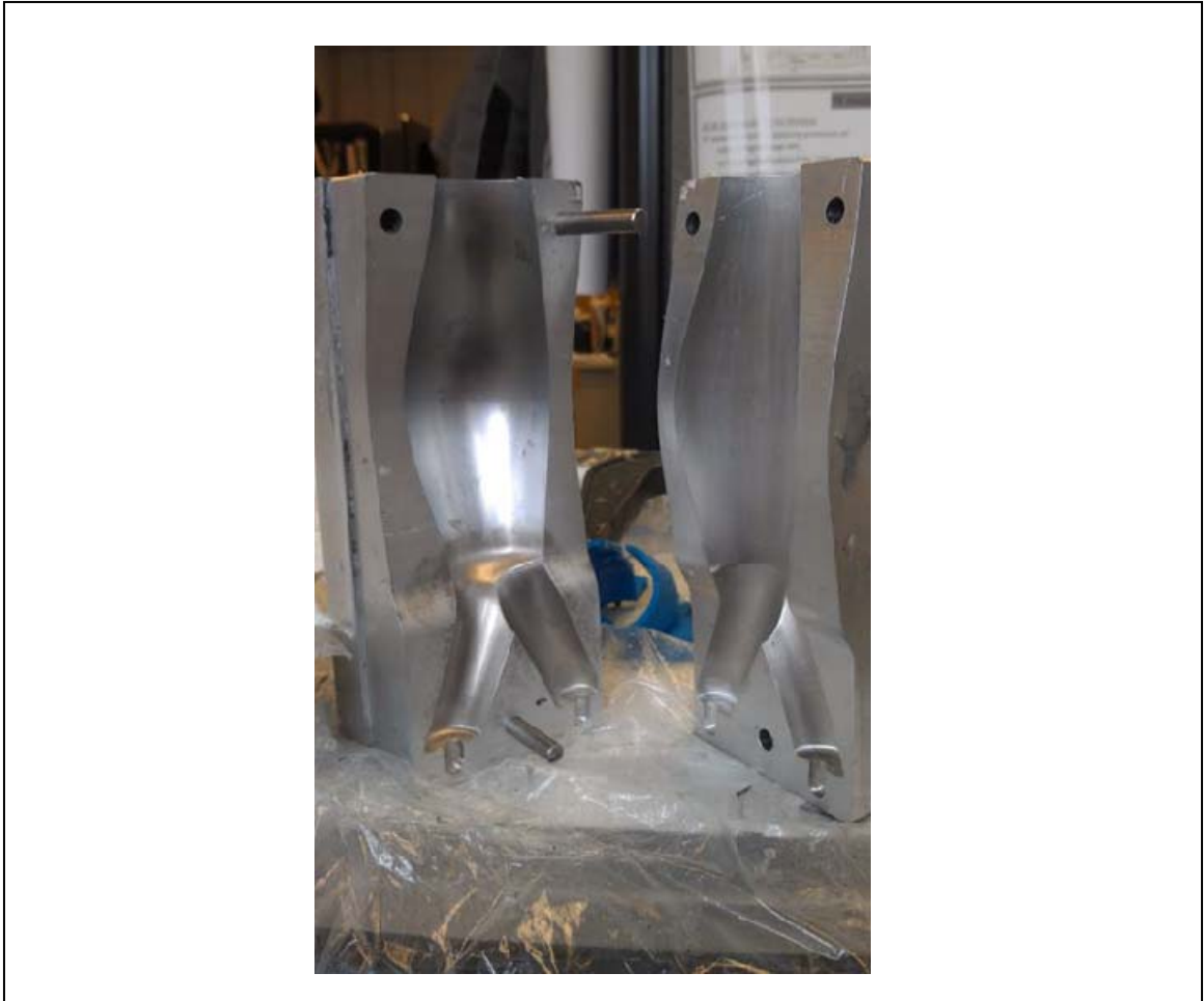
Figure 20: AAA mold aluminum blocks milled using a CNC machine. Dowel pins are used to ensure the two halves of the aluminum block are perfectly aligned.
